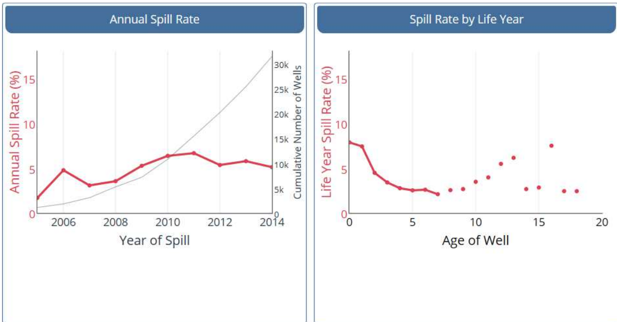
Figure 2 - Wastewater spill rates in the United States per number of wells in shale, coal and tight gas & oil operations. Data sourced from the National Center for Ecological Analysis and Synthesis spills data visualization tool: http://snappartnership.net/groups/hydraulic-fracturing/webapp/spills.html
