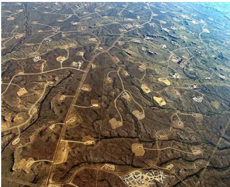
Figure 5: Dense well spacing in the U.S. state of Wyoming
