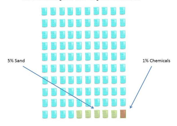
Shows the chemicals that are added to water to help hydraulic fracturing
