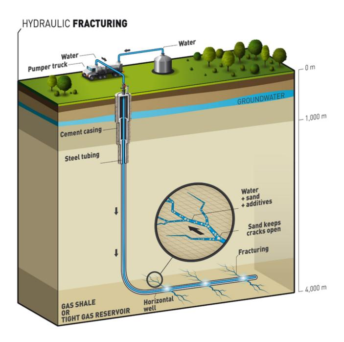
Shows how sand flows into the cracks in the shale rock and how gas flows out of the rock into the well.
