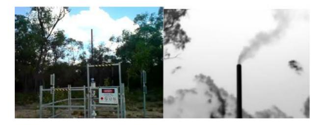
Visual and infrared images of continuous methane venting in the Queensland coal seam gas fields. February 2017
