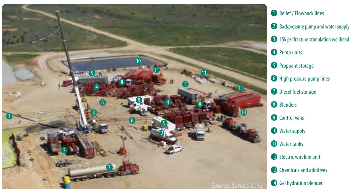
Figure 4.2: Well stimulation by hydraulic fracturing in Australia
