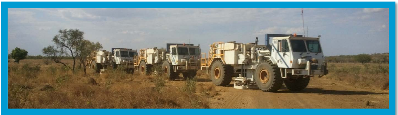
Figure 11: Vibroseis vehicles gathering seismic data
