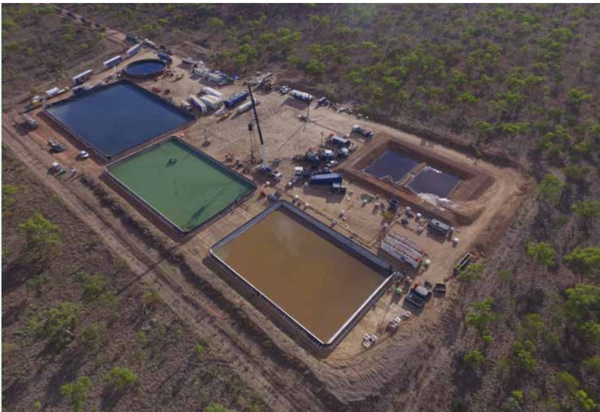
An aerial view of the Amungee NW-1H well site showing the above ground ponds during the flowback and production testing phase. Source: Origin.
