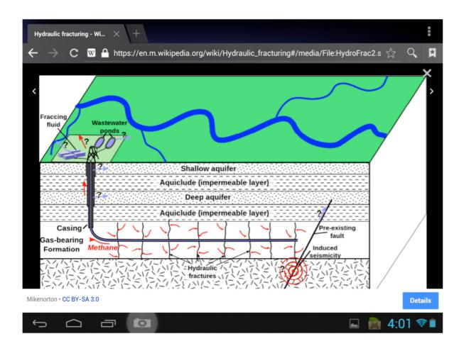
This picture is an example of how a fault can be in the effected area of fracking. The concentrated pressure from the high pressure injection and the fracturing of the shale will allow a passage along the fault line for contaminated fracking fluid and any acids or contaminants from mineralized zones that may be intersected to join into the aquifer or to the surface.
