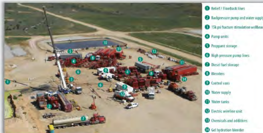
All equipment other than well head moved when drilling is completed
