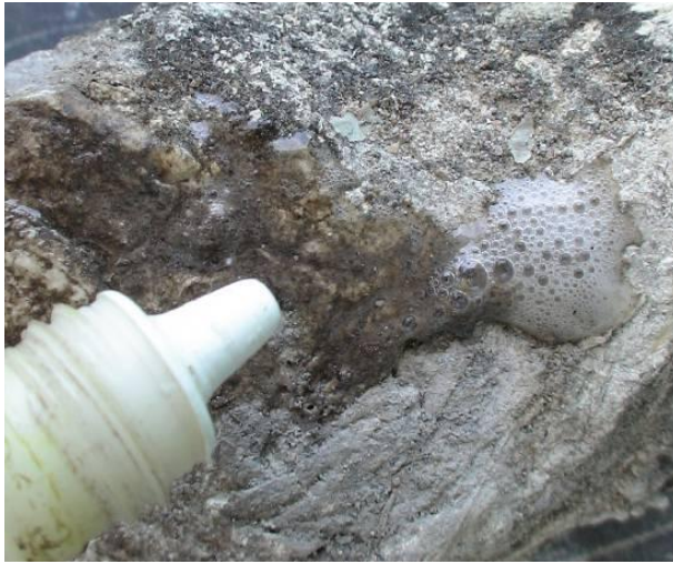
Plate 6.11 A drop of acid dissolving limestone as shown by the fizz. This is a common field test for carbonate rocks.
