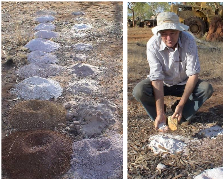
Plate 6.1 and 6.2 Sandstone drill cuttings from RN35869. Samples are taken every 3 m. Steve Tickell comparing drill cutting with rock outcrop of the same strata.
