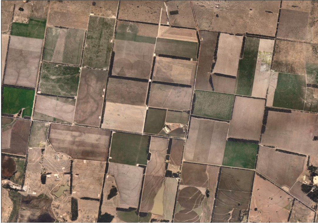
Figure 1.– Well sites coexisting with intense farming land (Surat Basin – NSW/Qld). This property contains 34 petroleum wells, identified by the small white boxes along property boundaries.
