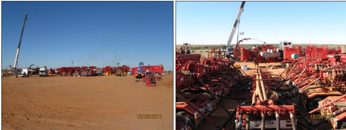
Plate 1: Fracture stimulation operations at Beach Energy's Holdfast-1 well (Cooper Basin) in 2011
