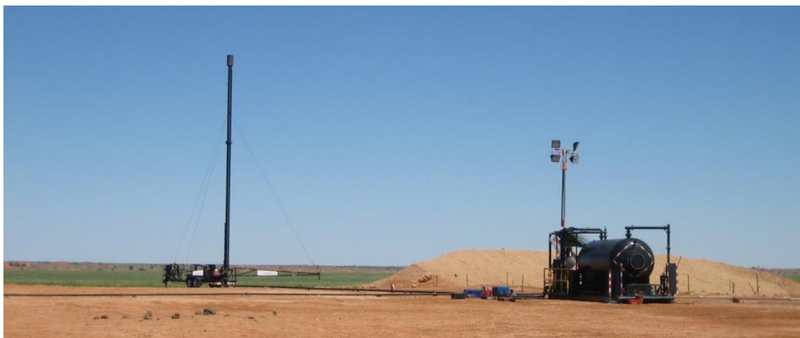
Figure 8: Separation and vertical flare set up in the Cooper Basin
