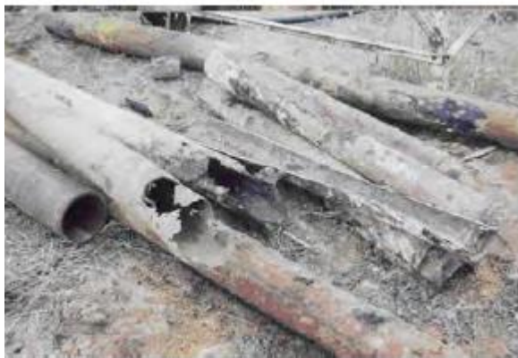
Figure 5 Examples of corroded casing (© Copyright, Mallee CMA 2005).
