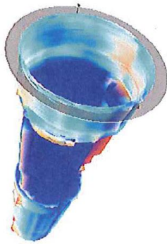
Figure 15 A 3D presentation of calliper data showing a damaged casing (dark blue) (© Copyright, Duguid & Tombari 2007 (modified); image courtesy of Schlumberger Limited).
