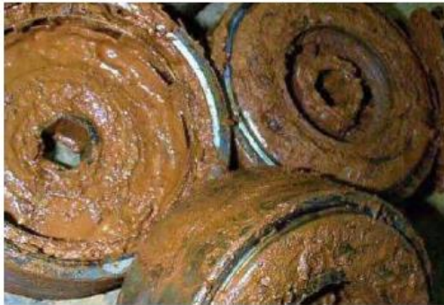
Figure 3 Example of iron fouling on a submersible pump (© Copyright, Forward 2008 in GHD 2010).
