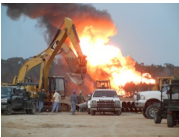
2011 Gas well blowout. It burned acres of forest in remote Village Creek State Park, Texas. Source: Nasti 2013
