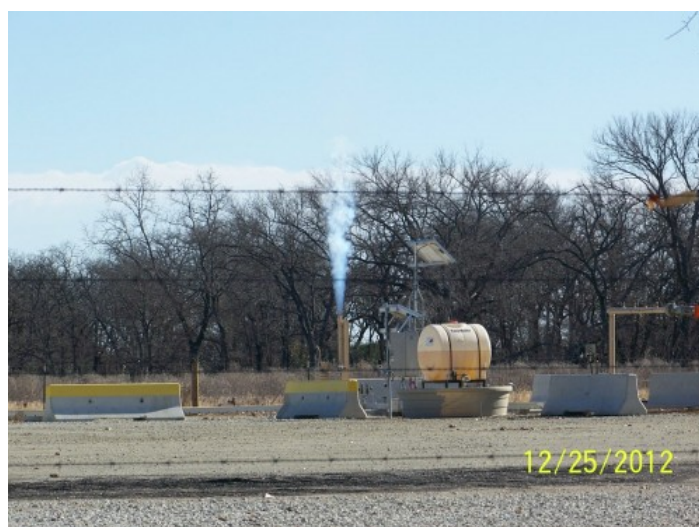
Figure 10. Venting shale gas containing toxic \text{H}_2\text{S} , Franklin, Texas. Source: Wilson 2012.
