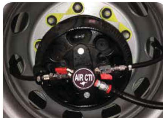
Purpose-built spray trucks have the ability to deflate their tyres to 18 psi (similar to pressures of tractor tyres) to reduce soil compaction. The truck then re-inflates the tyres on leaving the spray site so it can travel normally on public roads.
