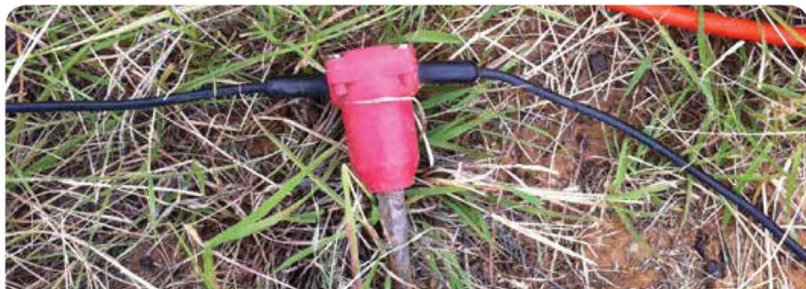
Geophone sensors with cables
