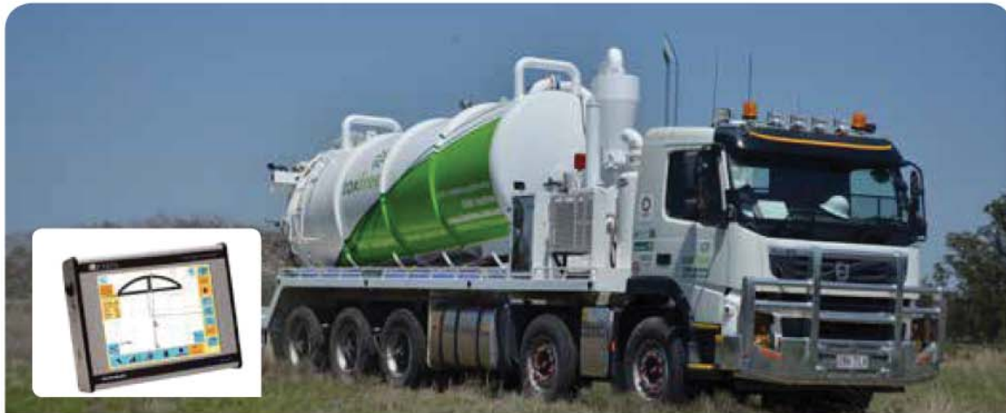
Precision GPS controls assist in assuring proper application rates, and proper application set back distances to environmentally sensitive areas and hazards.
