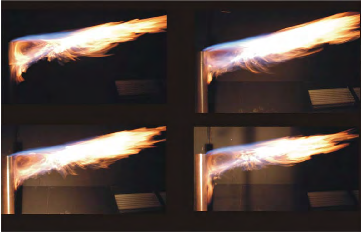
Figure 8.2: Visualization of 114.3 mm Flare Burning Natural Gas with an Exit Velocity of 0.4 m/s in a crosswind of 4 m/s.
