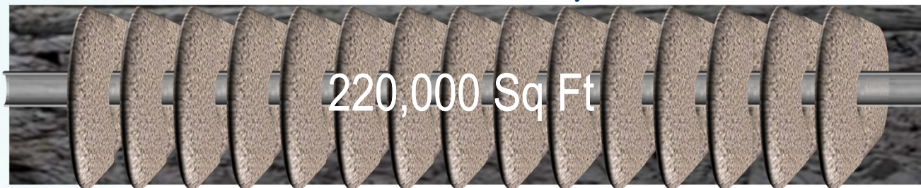
Horizontal, Perforated Well with 15 Hydraulic Fractures
