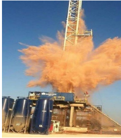
Pressurized lines being improperly connected or being hammered on while under pressure cause 'production fluid spills' Source: MEF n.d.
