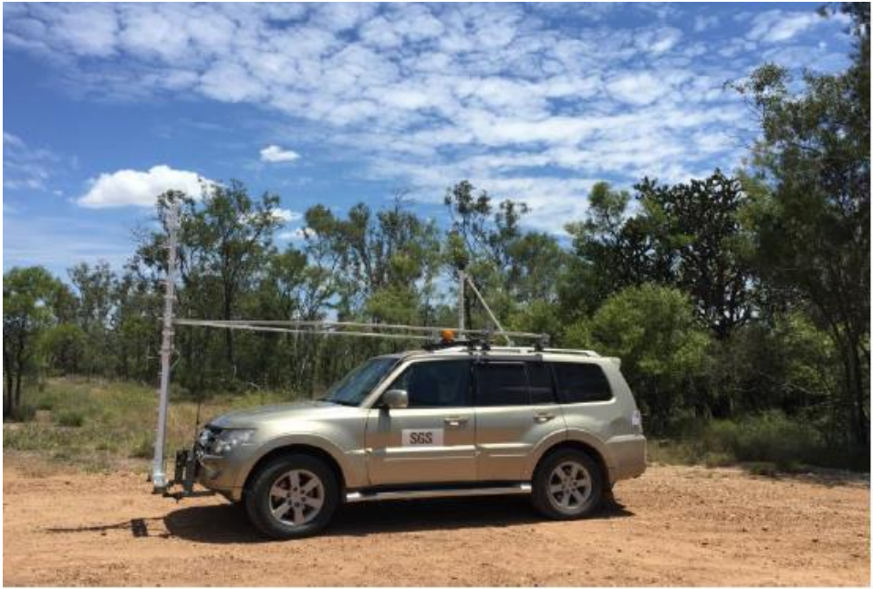
Figure 11.3 - Methane surveys using high precision cavity ring-down spectroscopy sensors to detect and quantify emissions sources across the Surat Basin (source Picarro)
