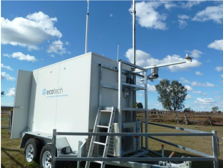
Figure 9.2 - Example of an air quality monitoring station within the Surat Basin
