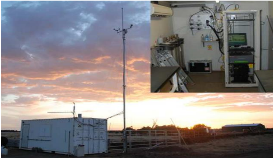
Figure 11.1 - GISERA Atmospheric GHG concentration monitoring station located on the Greenlea property on Origin's Ironbark tenure (Day, et al., 2015). These stations require access to power.
