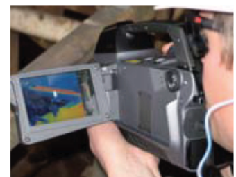
Tilttable, flip-out 4.3" High Contrast Color LCD allows you to view targets more safely from any angle.
