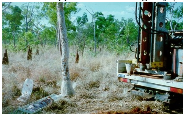
Plate 8 - Soil sampling with a small auger rig
