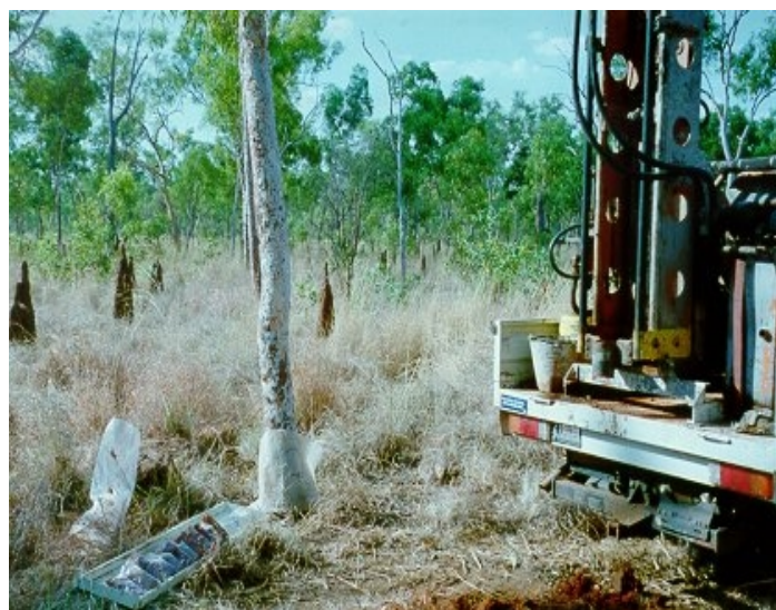
Plate 8 - Soil sampling with a small auger rig.
