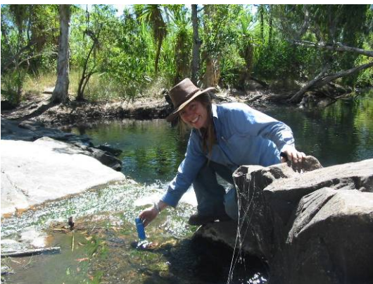
Plate 6.6 Ursula Zaar measuring the EC of Rosie Creek with an EC meter.
