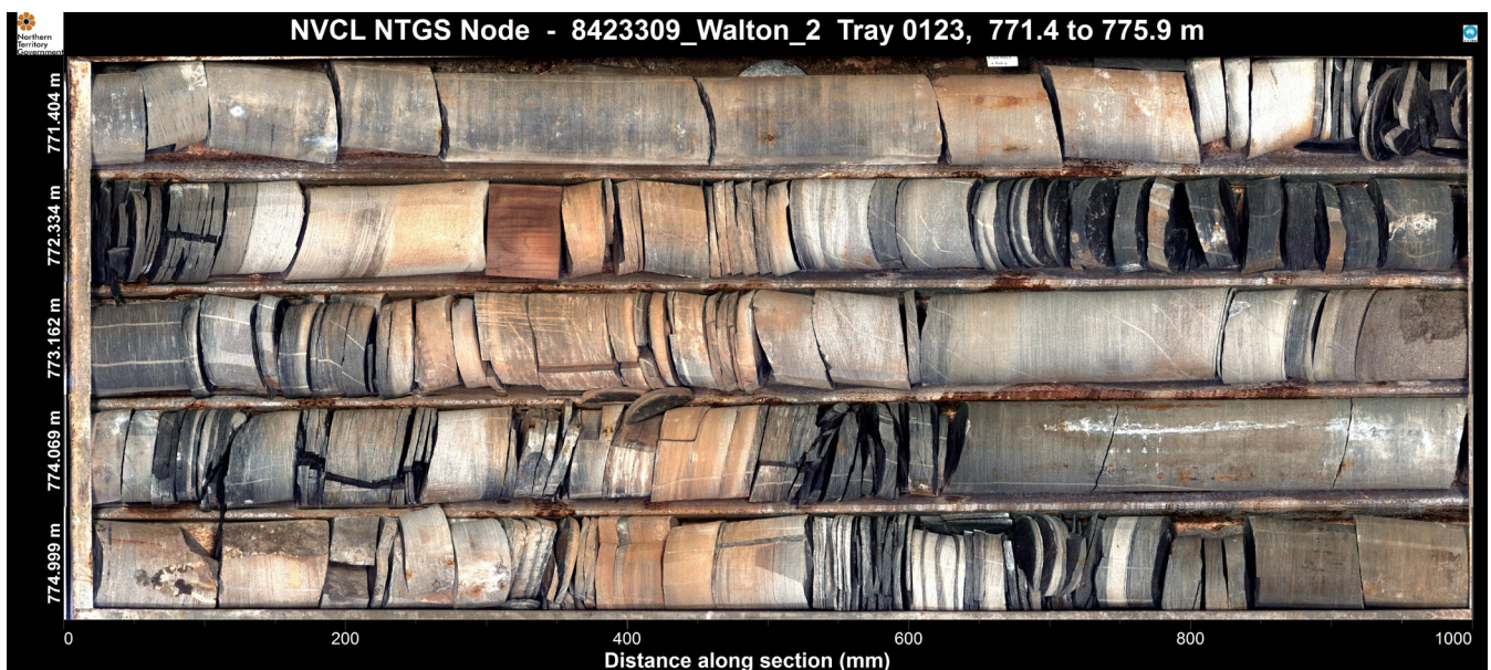
Figure 6. Lithological variability in lower Velkerri Formation (drill core from Walton 2: 771.4–775.9 m depth). Lighter coloured coarse clastic rocks are interbedded with darker, fine-grained siltstones on a centimetre scale.
