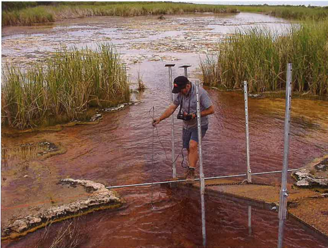
Pic: McDills – Flow gauging after platform constructed
