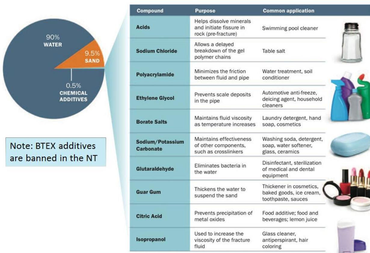
Figure 6: Typical hydraulic fracturing fluid additives that may be used. Source: Modified from US Department of Energy, 2009, Modern Shale Gas Development in the United States: A Primer.
