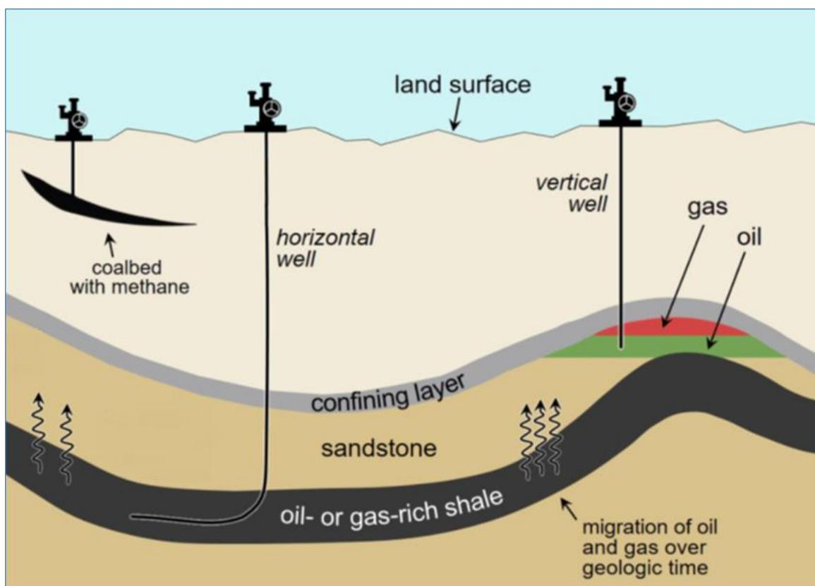
Figure 1: Schematic showing different types of petroleum accumulations and development Source: Modified from U.S. Environmental Protection Agency
