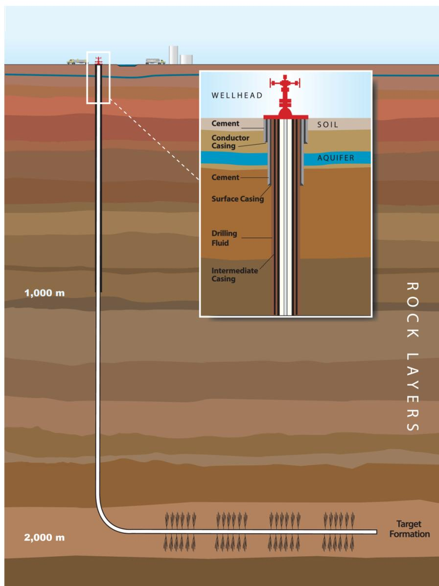
Figure 2: Schematic diagram showing typical well construction, casing, and horizontal drilling. Source: Modified from Society of Manufacturing Engineers.
