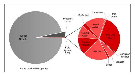
The functions served by the less than 1% of chemical additives used in a typical frac formulation include: increasing the viscosity of the fluid to improve proppant transport, reducing friction, inhibiting bacterial growth, preventing corrosion in the well casing and limiting the formation of scale and other precipitants that could impede the flow of oil and gas and fluids.
