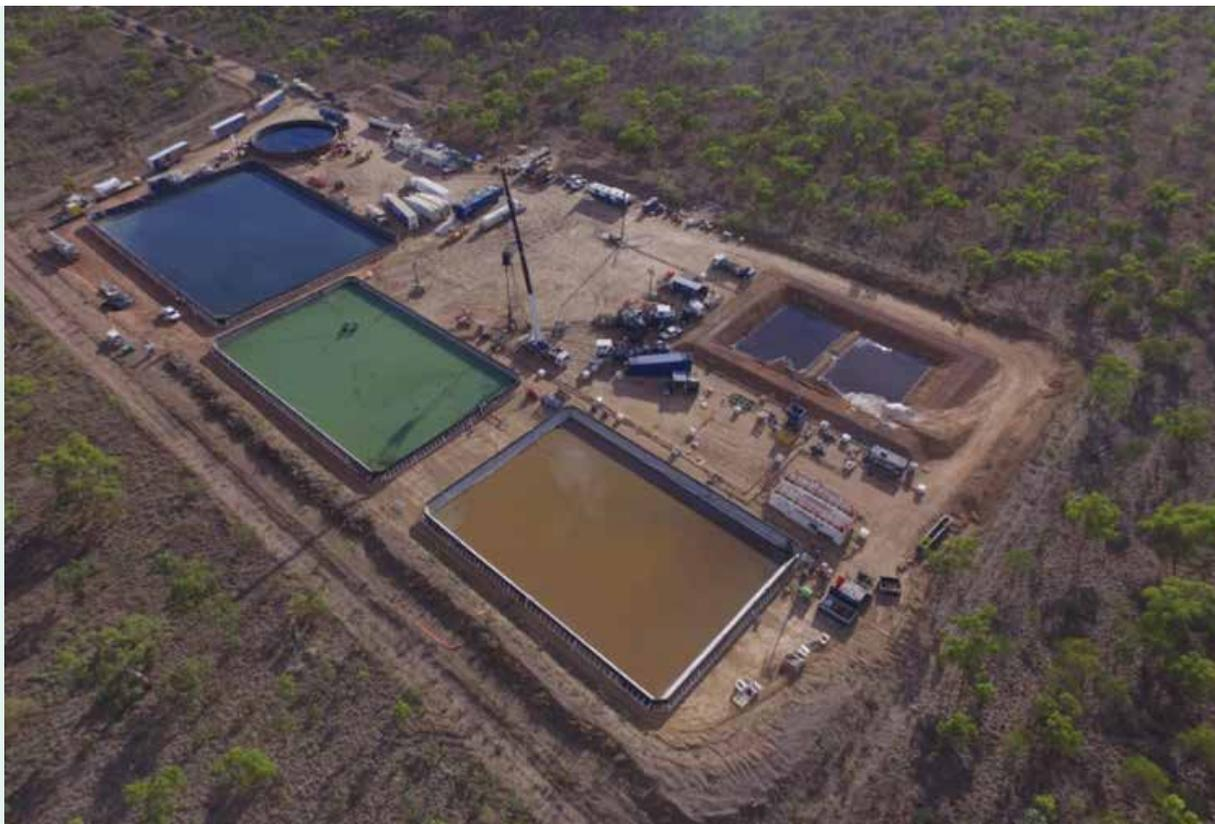
An aerial view of the Amungee NW-1H well site showing the above-ground ponds during the flowback and production testing phase. Source: Origin submission 153.
