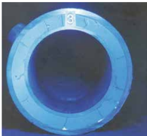
Figure 10: Cement sheath failure, resulting in cracks developing from pressure cycling on the internal casing. 58 Used with permission from the Society of Petroleum Engineers.
