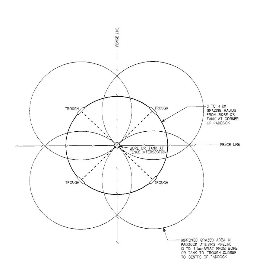
SKETCH SHOWING IMPROVED SIZE OF GRAZING AREA DUE TO PIPING AWAY FROM RELIABLE BORE OR TANK
