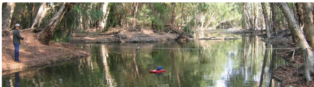
R. Metcalfe measuring the flow in the Roper River at Flying Fox Station with an Acoustic Doppler Current Profiler.
