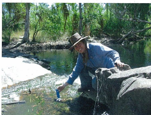
Plate 6.2 Ursula measuring the EC of a creek.
