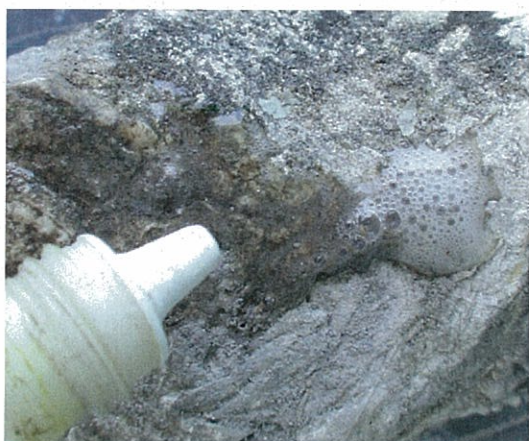
Plate 6.1 A drop of acid dissolving limestone as shown by the fizz. This is a common field test for carbonate rocks.
